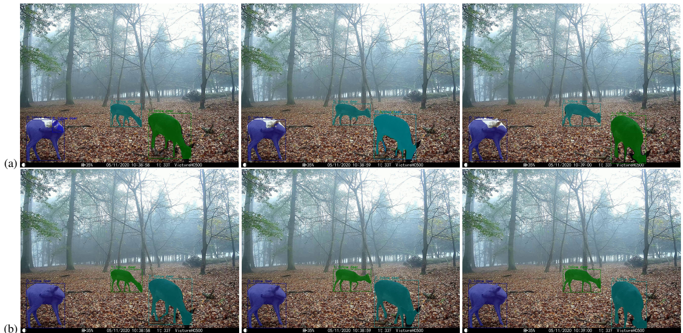
Fig. 3: Comparison of instance segmentation and tracking quality between Mask R-CNN + Tracktor++ (a) and SWIFT (b): Three frames of a video are displayed, each 1 second respectively 30 frames apart. Each found track is colored differently. [60]
